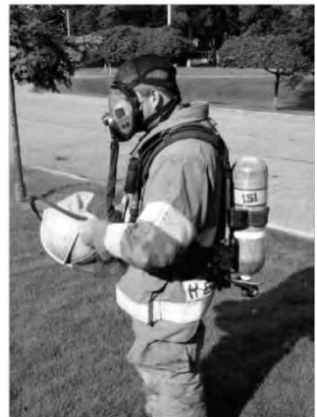
SCBA maintains positive pressure in the face piece at all times.
